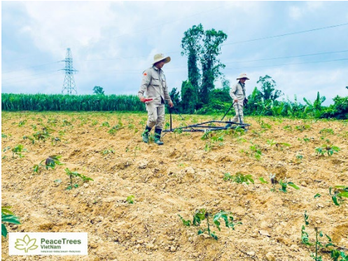
PeaceTrees Vietnam's technicians using mine detection equipment to locate unexploded ordnance in a cassava field in Quảng Bình province
